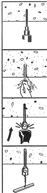
1. Drill a proper-sized diameter hole at a minimum depth (see chart on page 50, ANSI B212.15-1994).
