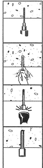
1. Drill a proper-sized diameter hole at a minimum depth (see chart on page 50, ANSI B212.15-1994).
