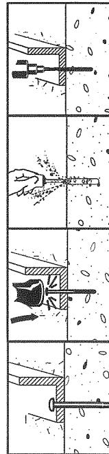
1. Drill a proper-sized diameter hole at a minimum depth (see chart on page xx, ANSI B212.15-1994).
