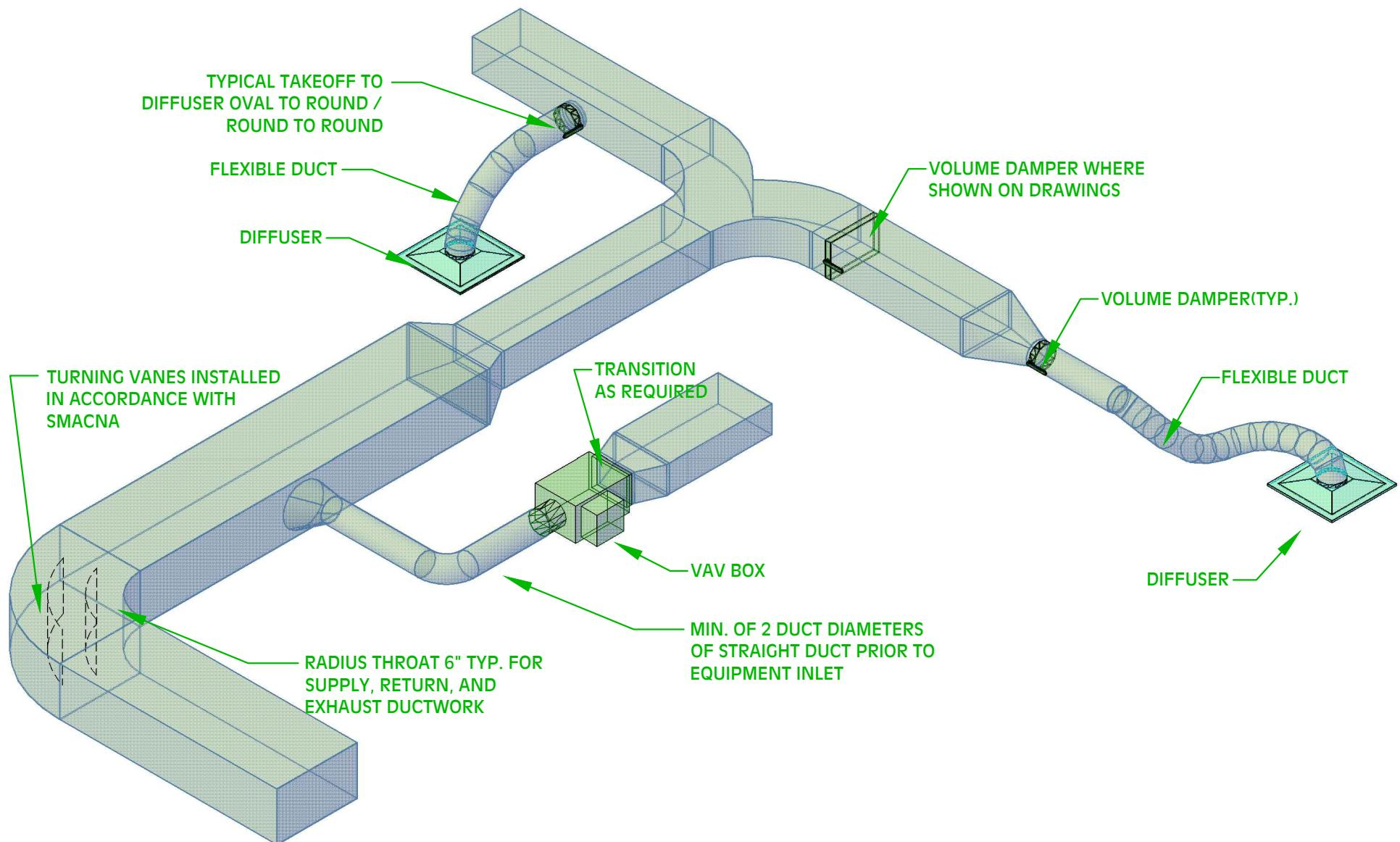
TYPICAL SUPPLY, RETURN AND EXHAUST DUCTS
