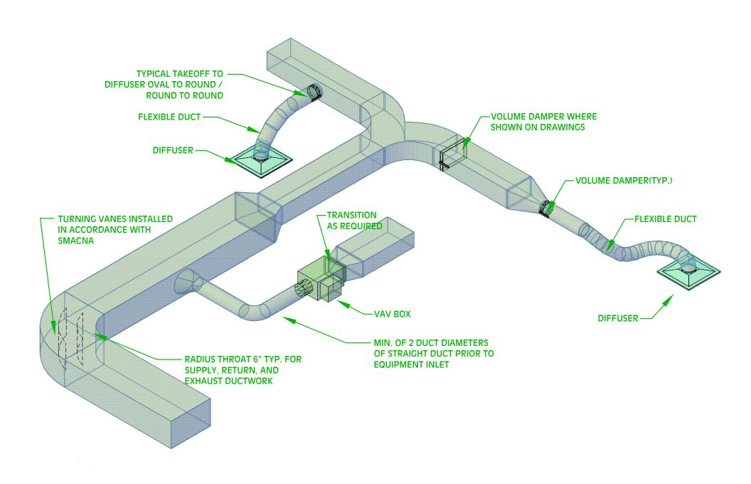
TYPICAL SUPPLY, RETURN AND EXHAUST DUCTS
